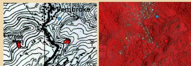
Figure 4. Sample of 1980's landslide locations (left) and the same points digitized over Ikonos image (right). Red dots represent verified landslide points. Blue points represent a control point.
